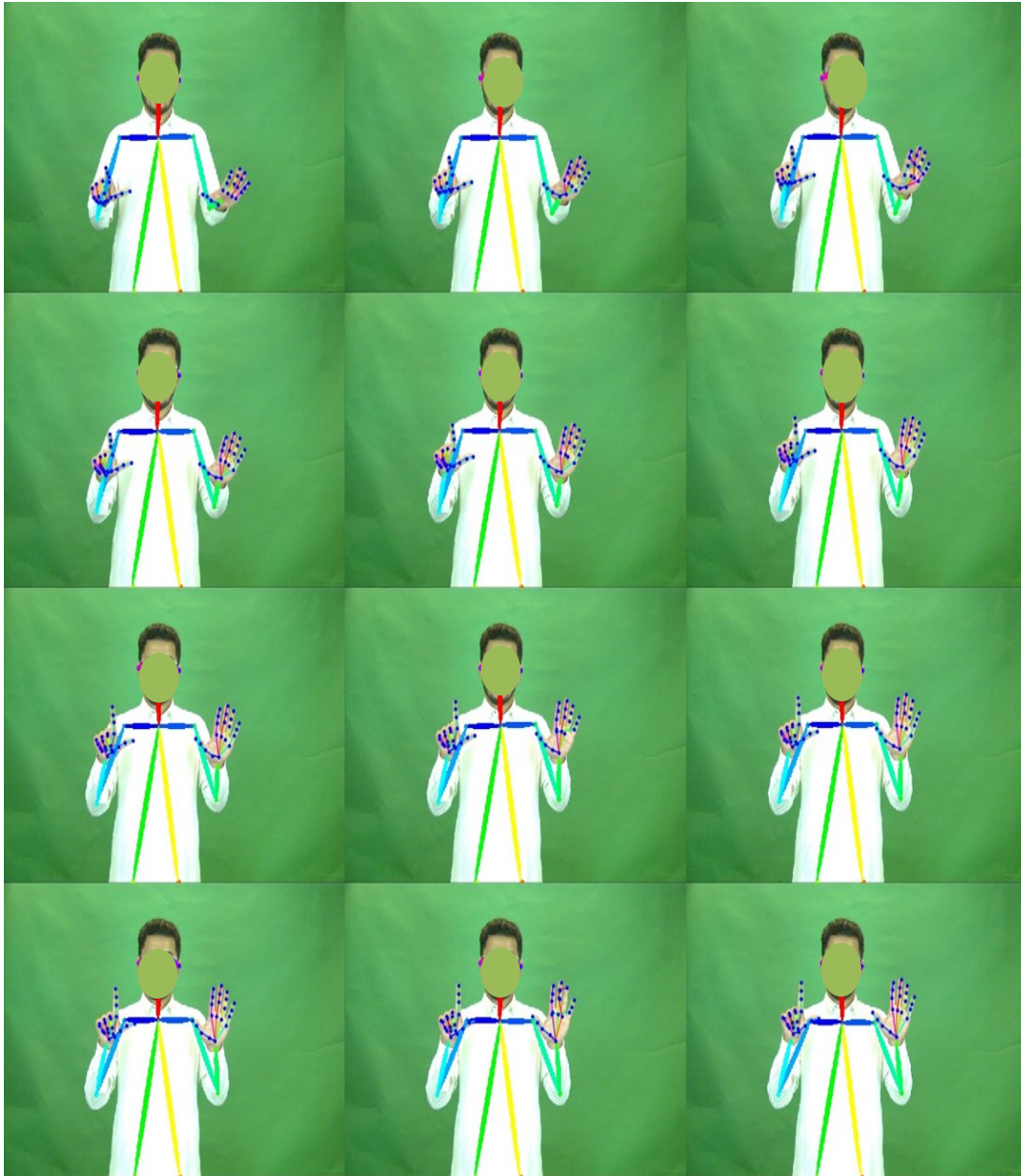
FIGURE 28, TWO HANDS + FINGER JOINTS DETECTION USING MEDIA PIPE LIBRARY IN KSU-SSL (SAMPLE 1)
