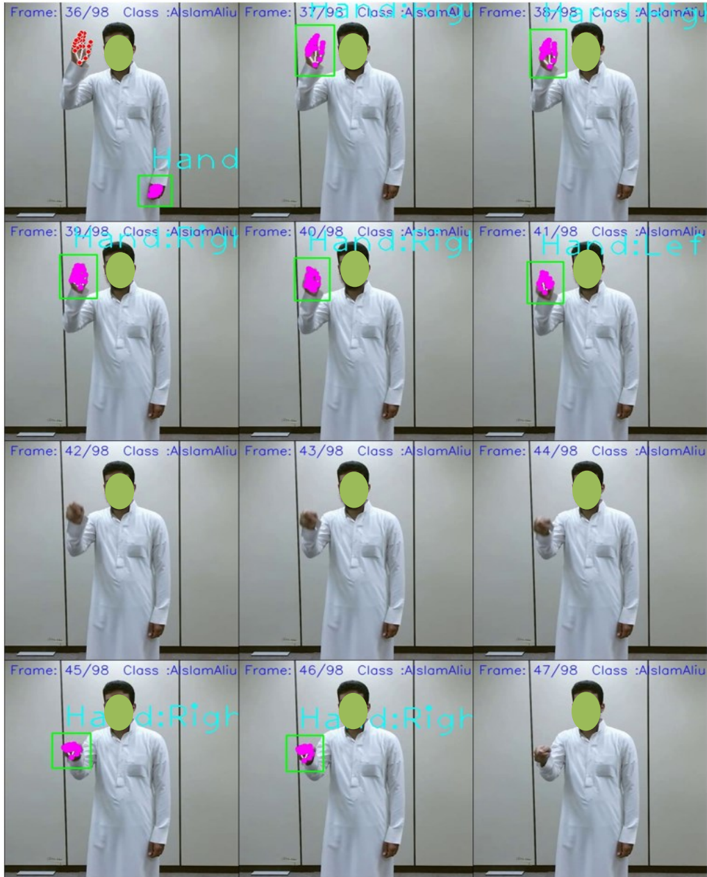
FIGURE 27, GOOGLE MEDIA PIPE HAND DETECTION OF A SECOND SAMPLE FROM THE KSU-ARSL
