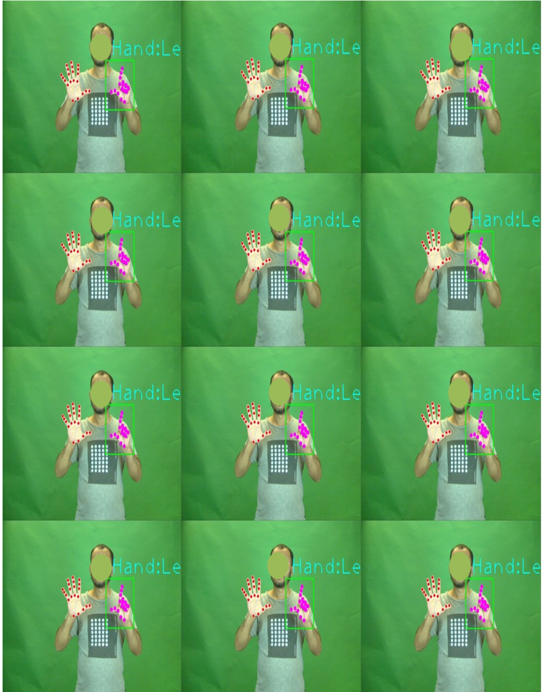
FIGURE 29, TWO HANDS + FINGER JOINTS DETECTION USING MEDIA PIPE LIBRARY IN KSU-SSL (SAMPLE 2)
